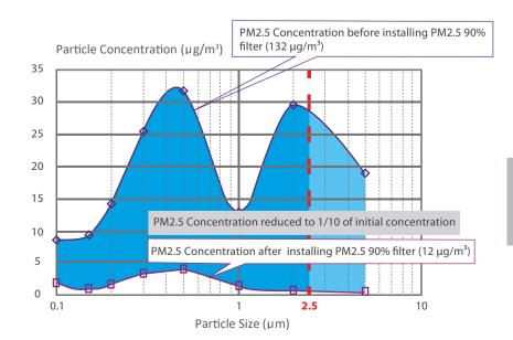
After installing the PM2.5 filter, average concentration of PM2.5 particles reduced to 1/10th
